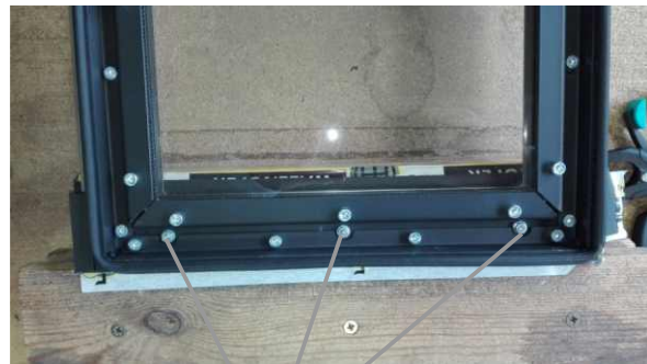
3 pcs. nuts (fixing stainless steel screen) above and below the glass pane
